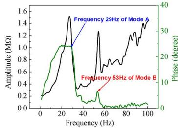
Fig. 3. Impedance–frequency testing results for the piezoelectric generator.
