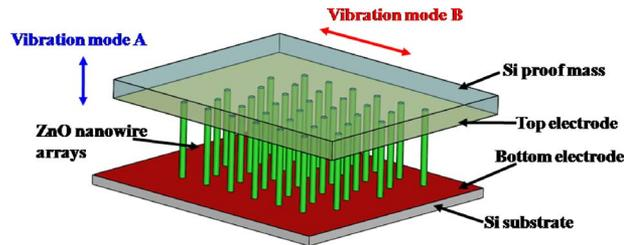
Fig. 1. Schematic diagram of the power generator, which consists of ZnO NWAs and Si proof mass for low-frequency-vibration harvesting. The generator is excited, and energy is scavenged by normal-mode A and shear-mode B.
