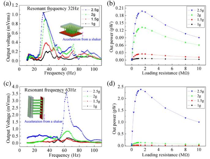
Fig. 4. (a) The output voltages of the generator when it is excited under different accelerations and resonant frequency of 32 Hz under normal-mode A. (b) The output power at 2.5-g acceleration and resonant frequency of 32 Hz under normal-mode A. (c) The output voltage of the generator when it is excited by different accelerations under shear-mode B. (d) The output power at 2.5-g acceleration and resonant frequency of 63 Hz under shear-mode B.
