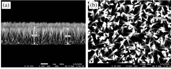
Fig. 2. (a) Cross-sectional SEM image of the self-aligned ZnO NWA grown by a chemical approach and having a length of 2.5  $\mu\text{m}$ . (b) SEM image viewed from the top of the self-aligned ZnO nanowire and having a single ZnO-nanowire diameter that varies from 53 to 75 nm.
