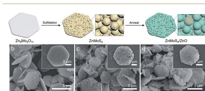
Fig. 1 (a) Schematic illustration of ZnMo compound synthesis. Low magnification SEM images of (b)  $\text{Zn}_5\text{Mo}_2\text{O}_{11}$ , (c)  $\text{ZnMoS}_4$  and (d)  $\text{ZnMoS}_4/\text{ZnO}$ , and the insets show their high magnification SEM images, respectively.
