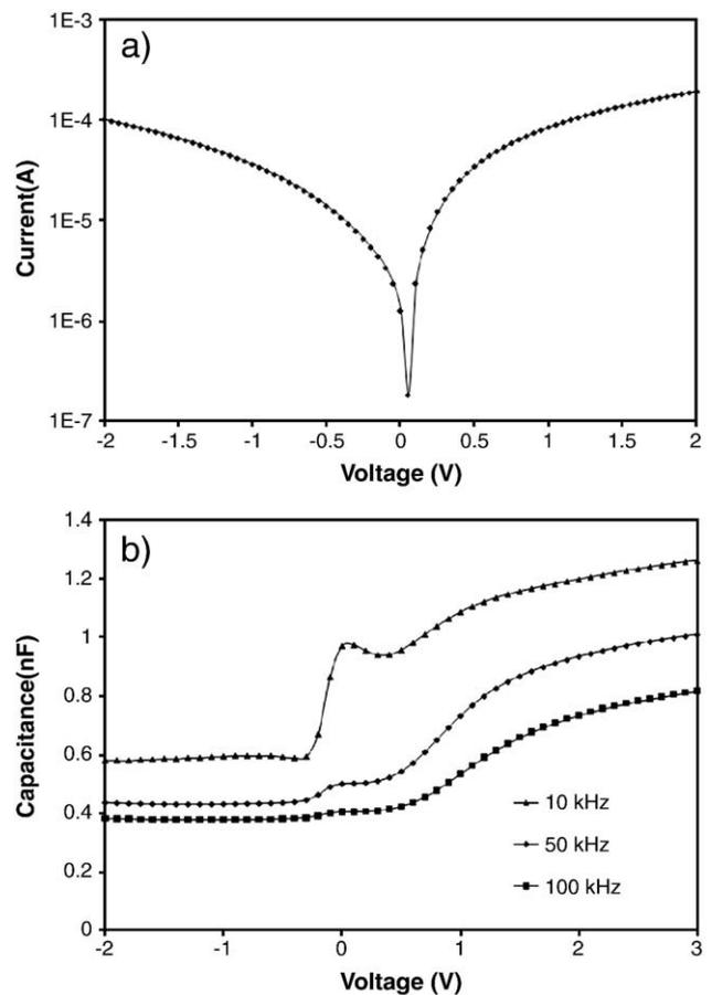
Fig. 6. Electrical measurements. a) *I*–*V* curve. b) *C*–*V* curves for 10, 50 and 100 kHz.
