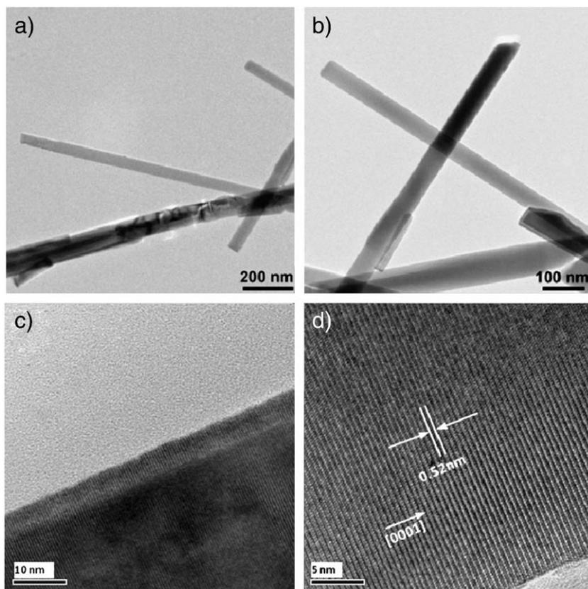
Fig. 3. TEM images. a) and b) Low magnification images of synthesized ZnO nanowires. c) and d) HRTEM images of the nanowire showing the [0001] growth direction and lattice spacing.
