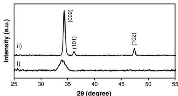
Fig. 1. XRD pattern of i) ZnO thin film (70 nm thickness) and ii) ZnO nanowire arrays.
