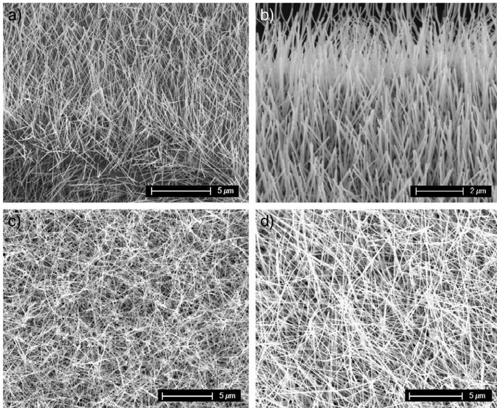
Fig. 2. SEM images show the morphologies of the as-prepared well-aligned ZnO nanowire arrays. a) Growth time of 30 min. b) Tilted view at 30°. c) Growth time of 2 h. d) Growth time of 3 h.
