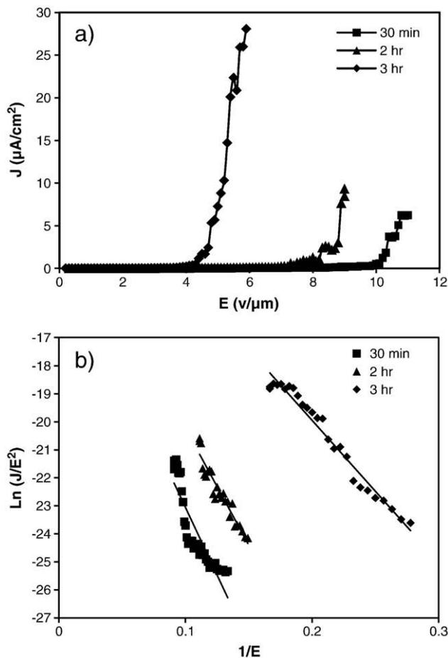
Fig. 5. Field emission properties of ZnO nanowire arrays: a) *J*–*E* plots. b) The corresponding *F*–*N* plots.
