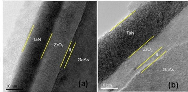
Fig. 5 HRTEM images of TaN/ $ZrO_2$ /epi-GaAs gate structure with PDA at (a) 400°C and (b) 500°C.
