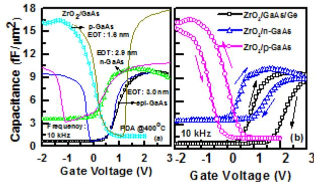
Fig. 2 (a) C-V characteristics of GaAs MOS capacitor at 10 kHz.  $ZrO_2$  (10nm) gate dielectric deposited on epi-GaAs and bulk-GaAs. (b) Hysteresis characteristics for the same gate stacks.
