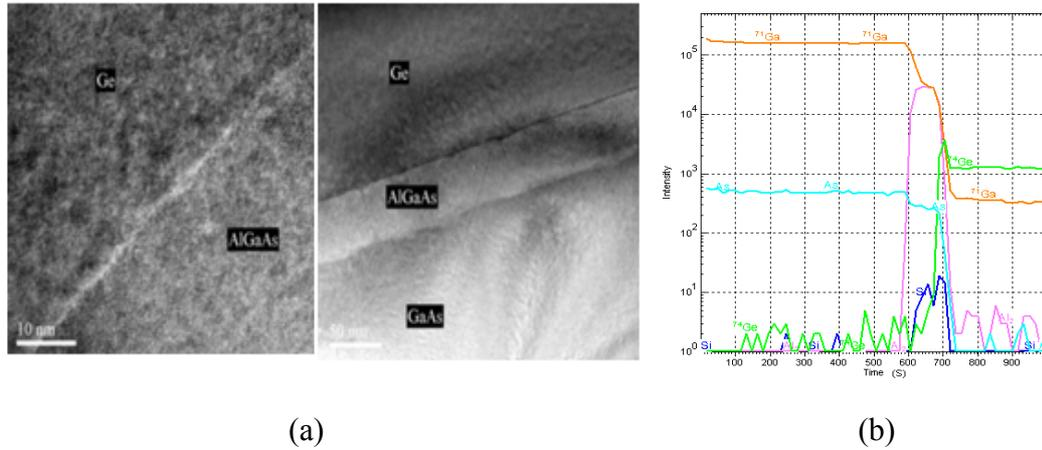
Fig. 1 (a) HR-TEM and (b) SIMS profiles of GaAs/Ge structure.
