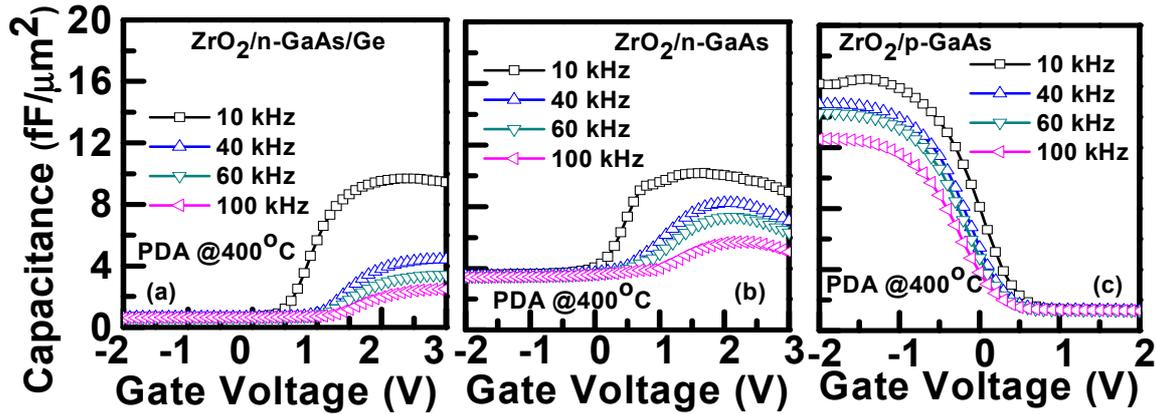
Fig. 3 Frequency dispersion in C-V characteristics between 10 kHz and 100 kHz for  $ZrO_2$  deposited on (a) epi-GaAs, (b) n-GaAs, and (c) p-GaAs, respectively and annealed at  $400^\circ C$ .
