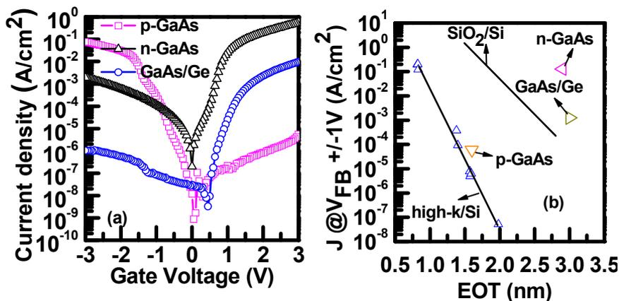
Fig. 4 (a) J-V Characteristics (b)  $J_g$  at  $V_{FB} \pm 1$  versus EOT of  $ZrO_2$  on epi-GaAs and bulk-GaAs.
