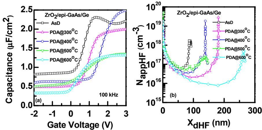
Fig. 6 (a) C–V characteristics for various PDA temperatures for 10nm thick  $ZrO_2$  on epi-GaAs. (b) Apparent doping profiles for the epi-GaAs obtained from MOS high frequency C–V characteristics.
