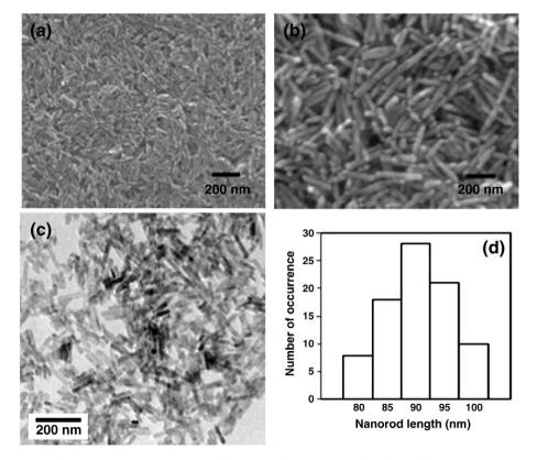
Fig. 1. (a-b) SEM and (c) TEM images of ZnO nanorods. (d) Histogram of the length of ZnO nanorods.
