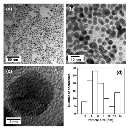
Fig. 2. TEM images of (a-c) low and high magnification and (d) histogram of the Au nanoparticles.
