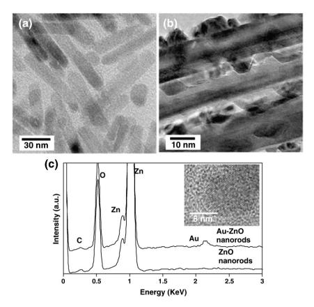
Fig. 3. TEM images of (a) as-synthesized ZnO nanorods and (b) ZnO nanorods with Au nanoparticles coating. (c) EDX spectra of pure ZnO nanorods and ZnO nanorods with Au nanoparticles coating (inset: High resolution image of the ZnO nanorod).
