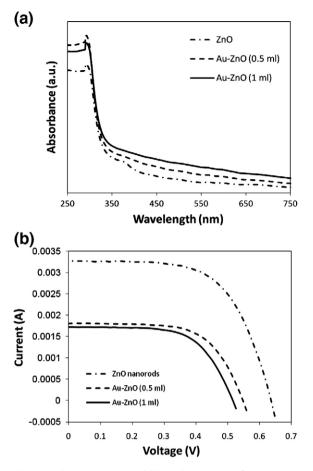
Fig. 4. (a) UV-vis absorption spectra and (b) I-V characteristics of DSSC using ZnO and Au-ZnO nanostructures.
